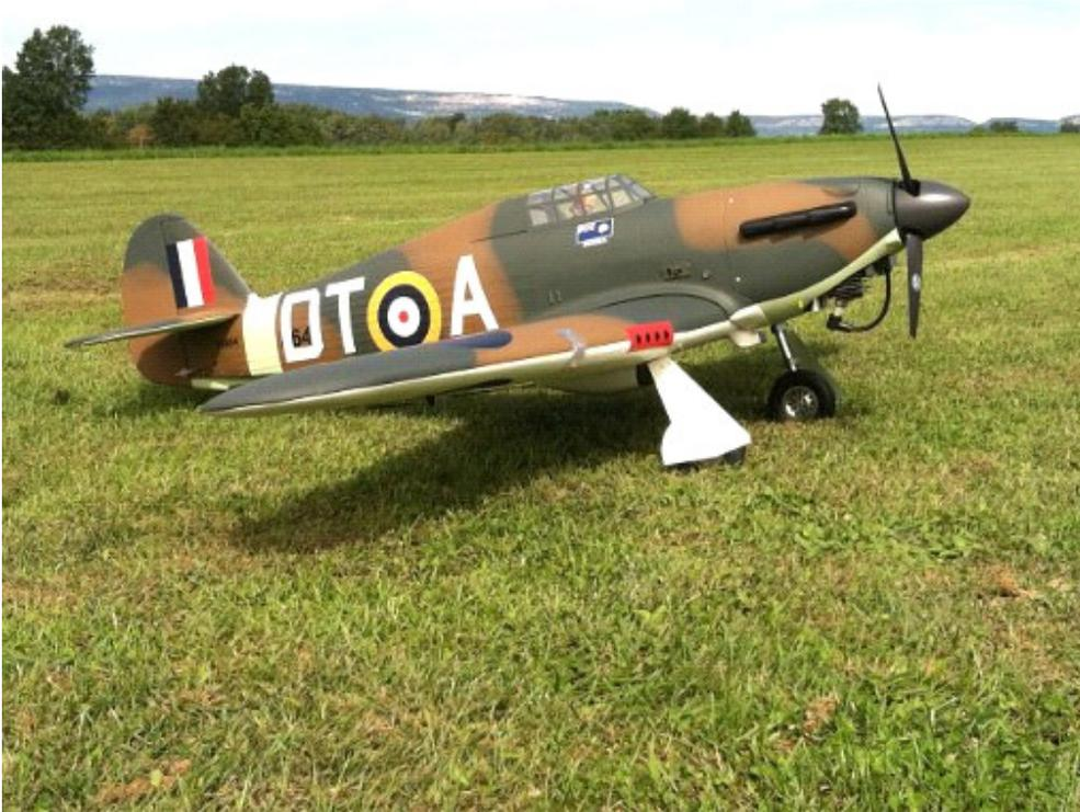
Bob reports: Test flew it earlier this summer and had to correct the balance and finally got time to fly it again. The model is an ESM Warbird ARF with 82" ws. I did have to modify the firewall significantly to wedge in the G-38 engine.
