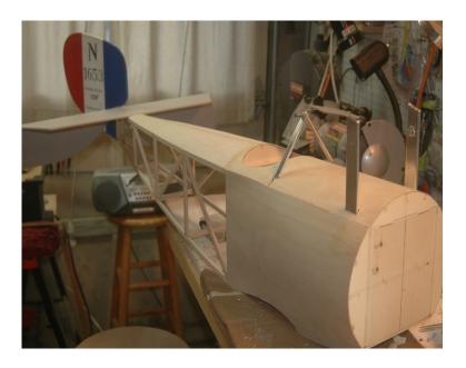
Here it is with the old flying stab attached and the old horizontal stab sitting on the fuselage. Fortunately on the first Nieuport I modified the attachment of the horizontal stab from gluing it on to using blind nuts and bolts.
