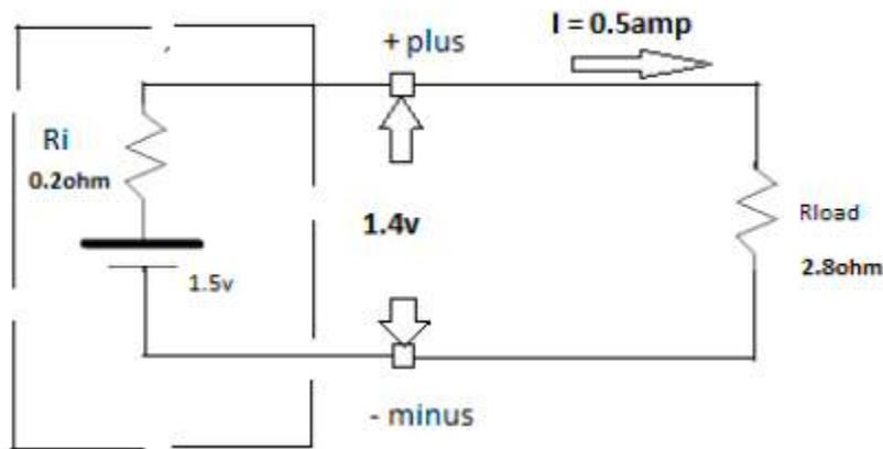
That 2.8ohm load resistor is in series with the INTERNAL RESISTANCE,  $R_i$ , of the cell. The total resistance is equal to the sum of all series resistance. Simply add  $R_i + R_l$ ,  $0.2+2.8 = 3.0\text{ohms}$  total. Now go back to Ohm's Law, using the form  $I = E/R$ , and you get  $1.5\text{v}$  divided by  $3.0\text{ohms} = 0.5\text{amp}$ . Its that 0.2ohm INTERNAL RESISTANCE that causes the output voltage to drop down to 1.4v. Look
