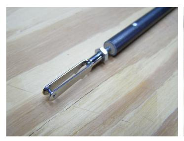
This end of the carbon fiber tube has a 4-40 threaded clevis and jam nut attached. You can see the wood plug well here.
