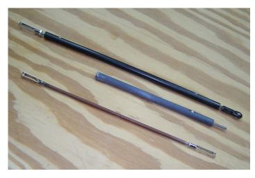
The top two push rods are carbon fiber tubing with wood "plugs" inserted and epoxied into each end to capture an "L" shaped 4-40 rod..
