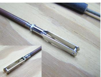
One end of the 1/8 steel rod has been threaded for a 4-40 clevis and also has a jam nut. The opposite end has been turned down and a solder style clevis attached.
