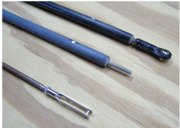
The bottom push rod is 1/8 dia steel welding rod. It is copper clad for rust prevention and weldability. It is also very easy to solder and machine yet this material is extremely stiff and perfect for our applications. I use this type of push rod for all my aileron set-ups..
