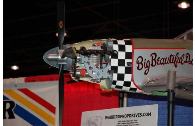
Warbird Prop Drives. It's a four-blade, constant speed gear drive for a 50cc gasser. Constant speed means that a servo and sensor adjusts the pitch of the prop in flight in response to the throttle and airspeed! I'll take two please. Sig and Balsa USA and a horde from Hobbico/Great Planes were there as well as all the engine and radio manufacturers.
