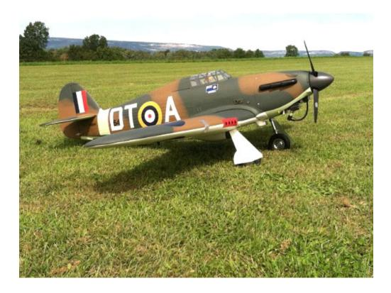
Bob reports: Test flew it earlier this summer and had to correct the balance and finally got time to fly it again. The model is an ESM Warbird ARF with 82" ws. I did have to modify the firewall significantly to wedge in the G-38 engine. It flies very nice.
