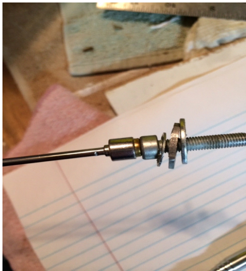
The bolt and washers on the magnet. On final installation, only a washer will be installed on the inside.
