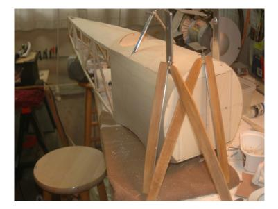
The wing struts are stained and I plan to varnish them next. The cabane struts are covered with aluminum tape that I got at Lowes.
