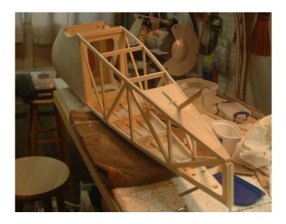
The Nieuport getting its tail skid. This is just the beginning of the process. On the first one, the tail skid built per plans was very easily knocked lose due to lateral pressure on it when the plane was turned on the runway. The whole structure is quite large so I beefed that one up with plywood side supports and a quarter square hardwood rail on both sides of the side supports for a larger footprint on the fuselage.
