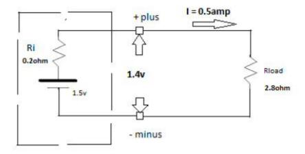
That 2.8ohm load resistor is in series with the INTERNAL RESISTANCE, Ri, of the cell. The total resistance is equal to the sum of all series resistance. Simply add Ri + Rl, 0.2+2.8 = 3.0ohms total. Now go back to Ohm's Law, using the form I = E/R, and you get 1.5v divided by 3.0ohms = 0.5amp. Its that 0.2ohm INTERNAL RESISTANCE that causes the output voltage to drop down to 1.4v. Look
