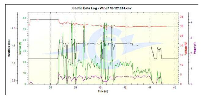
I've only selected Throttle, Current, Voltage and Ripple to keep this easily seen. Notice how the Voltage (displayed in red) drops as the flight progressed, the ripple was changing and Current varied widely with changes in Throttle setting.
