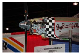
Warbird Prop Drives. It's a four-blade, constant speed gear drive for a 50cc gasser. Constant speed means that a servo and sensor adjusts the pitch of the prop in flight in response to the throttle and airspeed! I'll take two please. Sig and Balsa USA and a horde from Hobbico/Great Planes were there as well as all the engine and radio manufacturers.
